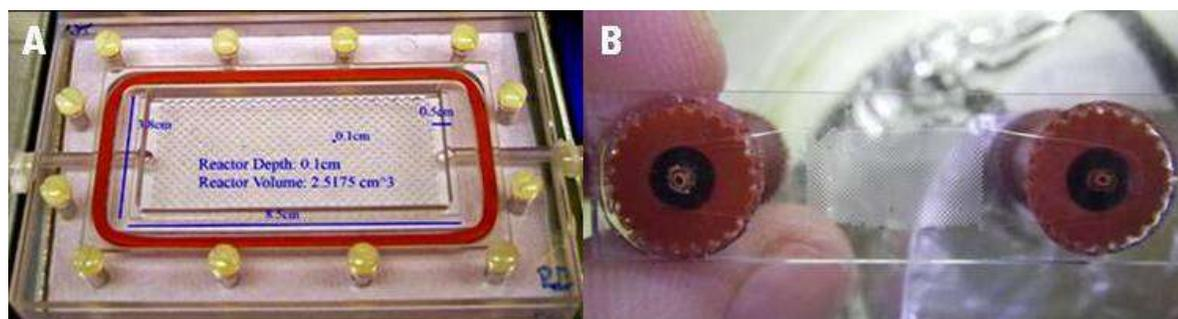
**Figure 1** - (A) 2D porous media reactor with 1mm pore structures. (B) 2D porous media reactor with 100µm pore structures designed for CSLM imaging.
