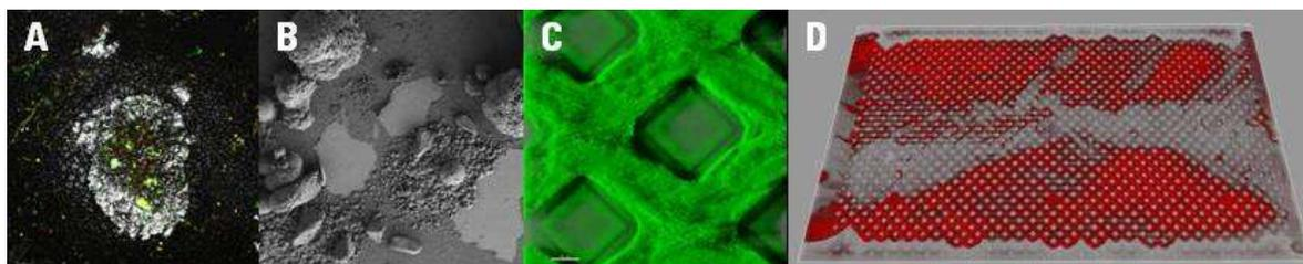
**Figure 2** – (A) CSLM image of a microbially induced  $\text{CaCO}_3$  crystal (gray) with cells attached (green and red). (B) FEM micrograph of microbially induced  $\text{CaCO}_3$  precipitation. (C) Living bacterial biofilm grown in a porous media reactor with  $100\mu\text{m}$  pore structures. The bacterial strain is expressing green fluorescent protein, so no staining was required. (D) 3D CSLM reconstruction of a stained bacterial biofilm grown in the reactor pictured in Fig 1B.
