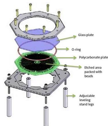
**Figure 1.** Radial Flow Reactor used to study MICP.
