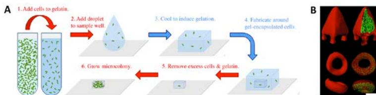
**Figure 1:** (A) Schematic depicting *in situ* fabrication around cells encapsulated in gelatin. The red and blue arrows indicate steps performed at 37°C or 18–22°C, respectively. (B) Fluorescence isosurfaces show *P. aeruginosa* microcolonies within a surface-anchored 2-pL pyramid (top) and a 3-pL torus (bottom). Scale bar, 20  $\mu\text{m}$ .
