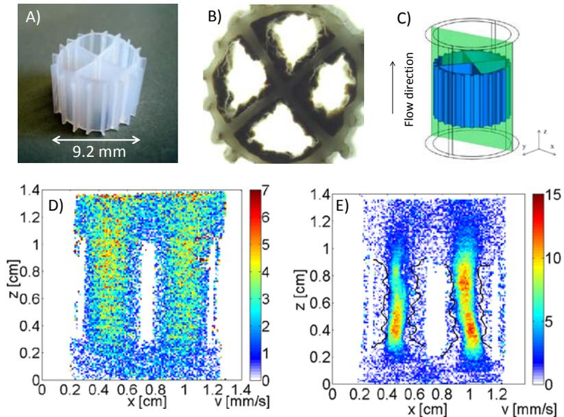
**Figure 1.** Carrier material type K1 (AnoxKaldnes, Sweden): **A)** clean carrier, **B)** cultivated carrier, **C)** setup for flow experiment. Flow velocity maps (axial plane indicated as green layer in C): **D)** clean carrier, **E)** cultivated carrier, where the black lines indicate the biofilm surface.
