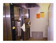
An autoclave is a specialized piece of equipment designed to deliver steam generated heat under pressure to a sealed chamber, with the goal of decontaminating or sterilizing its contents.
