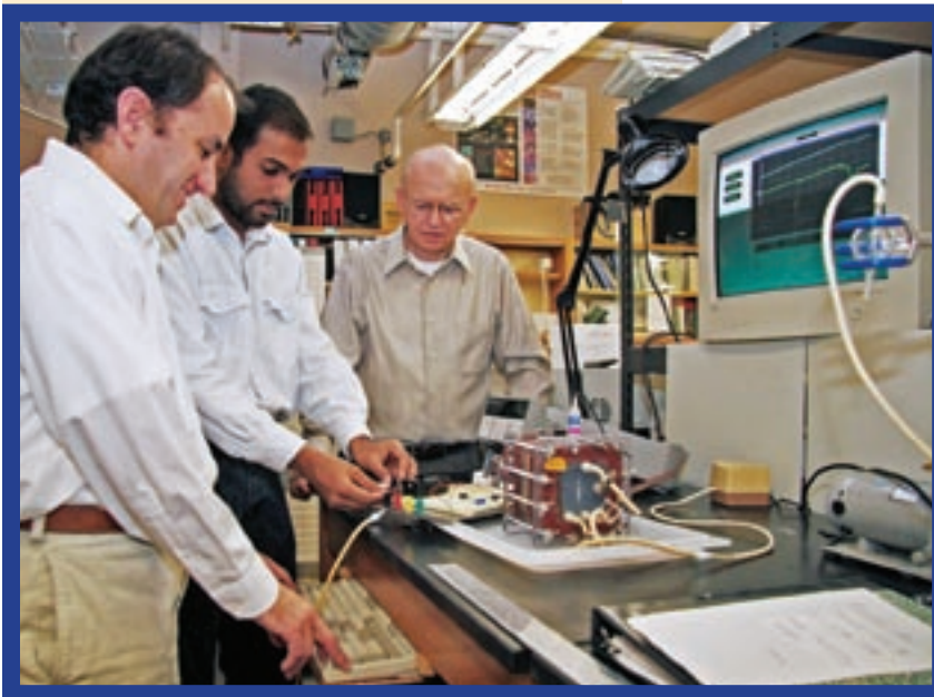
Raaja Raajan Angathevar Veluchamy (center), MS, environmental engineering, measures the electrical power generated by a microbial fuel cell that the team operates in the lab while Haluk Beyenal (left) and Zbigniew Lewandowski (right) look on.
